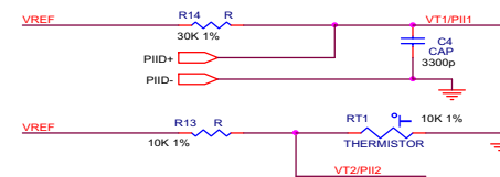
TEMPERATURE SENSING CIRCUIT
