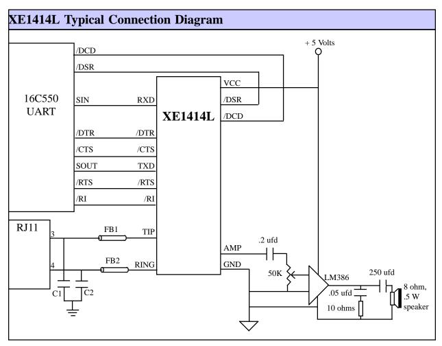
Note: RJ11 Pin assignments reflect a 6-pin connector. Tip and Ring are always the center pins of the RJ11 Jack.
