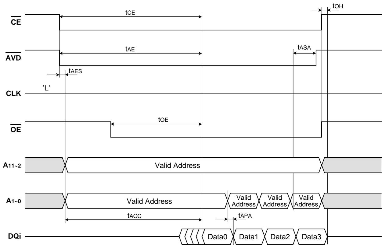
**Synchronous Burst Read Operation**
