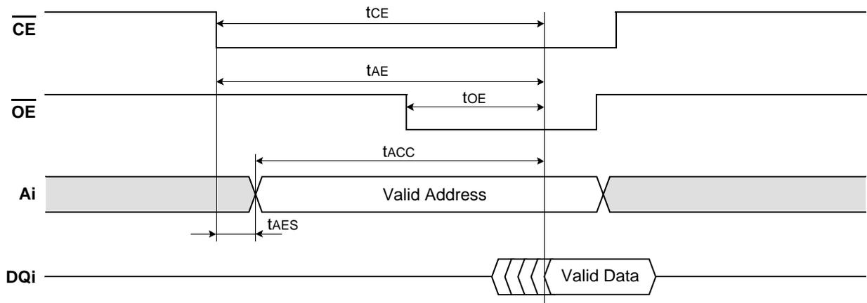
**Latched Asynchronous Read Operation**
