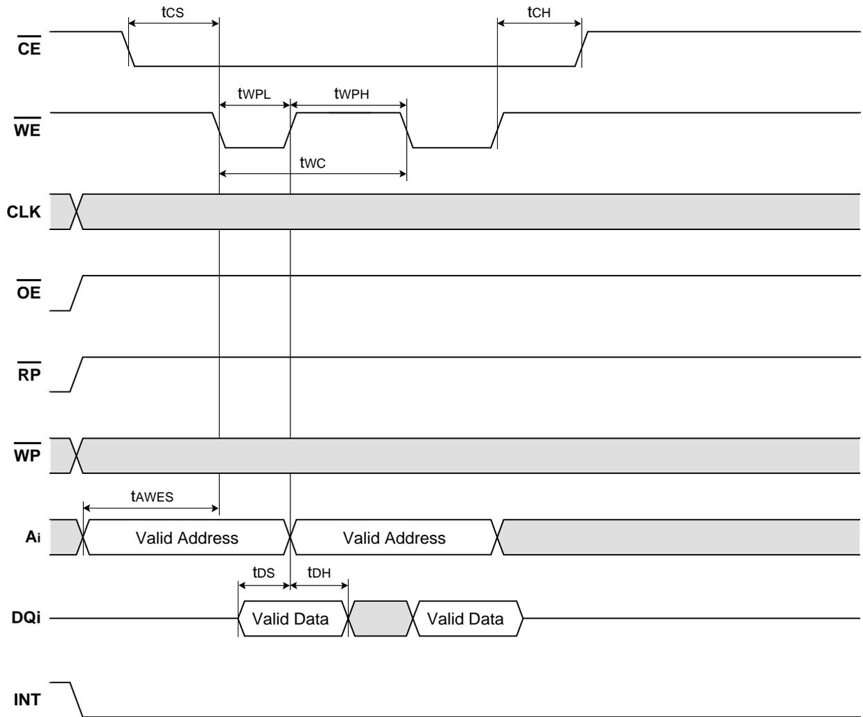
Figure 6. Latched Asynchronous Write Mode
