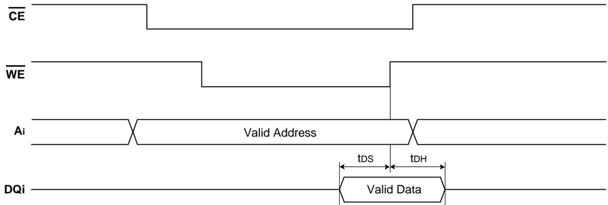
**Latched Asynchronous Write Operation**
