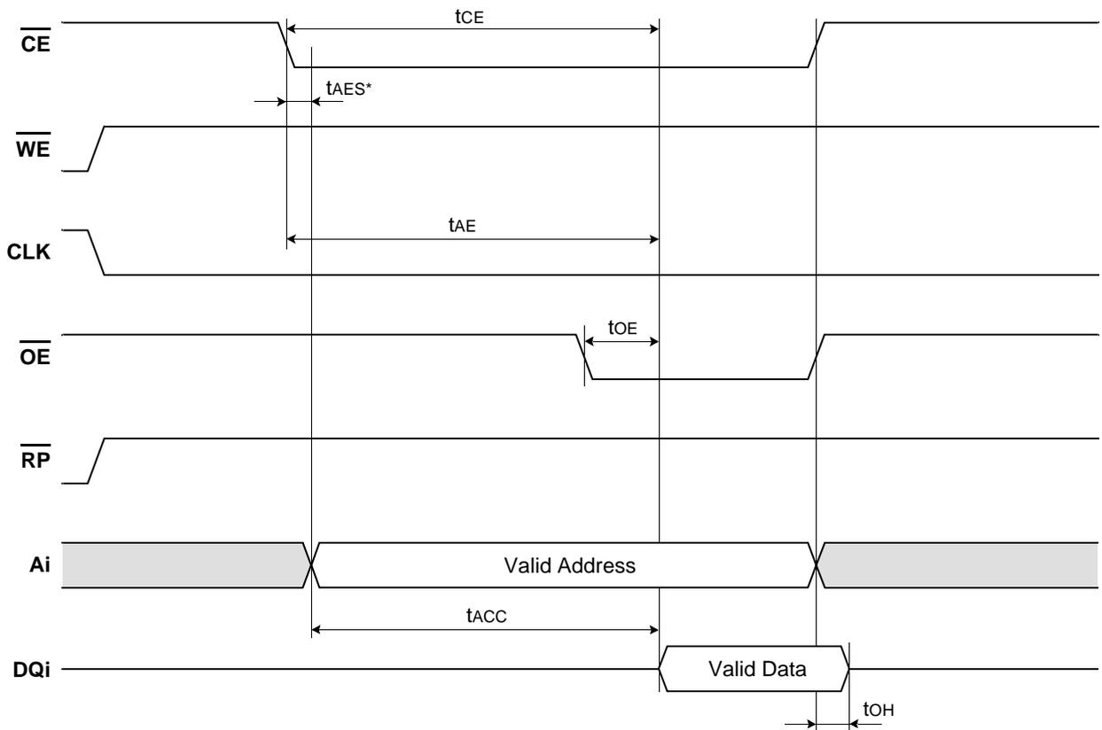
Figure 2. Latched Asynchronous Read Mode
