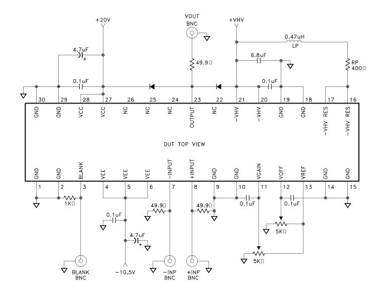
The connection circuit shown above is for the MSK 1903-0 evaluation board. The Rp and Lp are external components and must not be located near ground planes if possible. A high quality resistor such as Bradford Electronics P/N FP10-400 is required for optimum response times. Use an inductor with a high self-resonant frequency that can withstand the currents required for the application.
