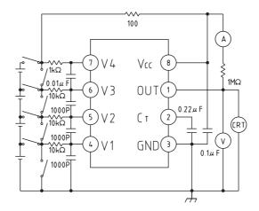
Note: By shorting each cell, two-, three- and four-cell series can be accommodated. A V4 cell should always be connected. If the V4 cell is shorted, the chip may not function correctly.
