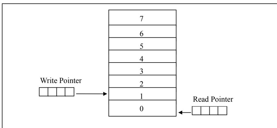
**Figure 5. Transmit FIFO Outline (example for 8 bytes FIFO)**
