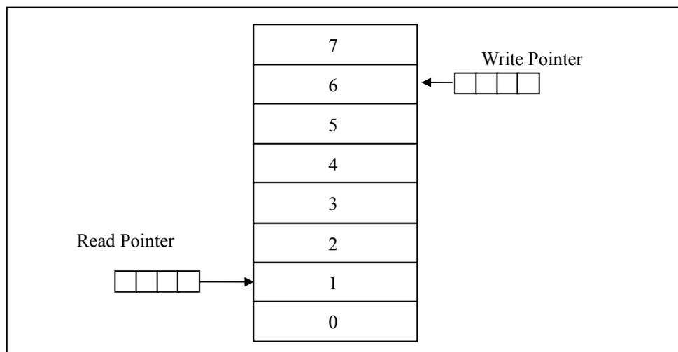
**Figure 6. Receive FIFO Outline(example for 8 bytes FIFO)**
