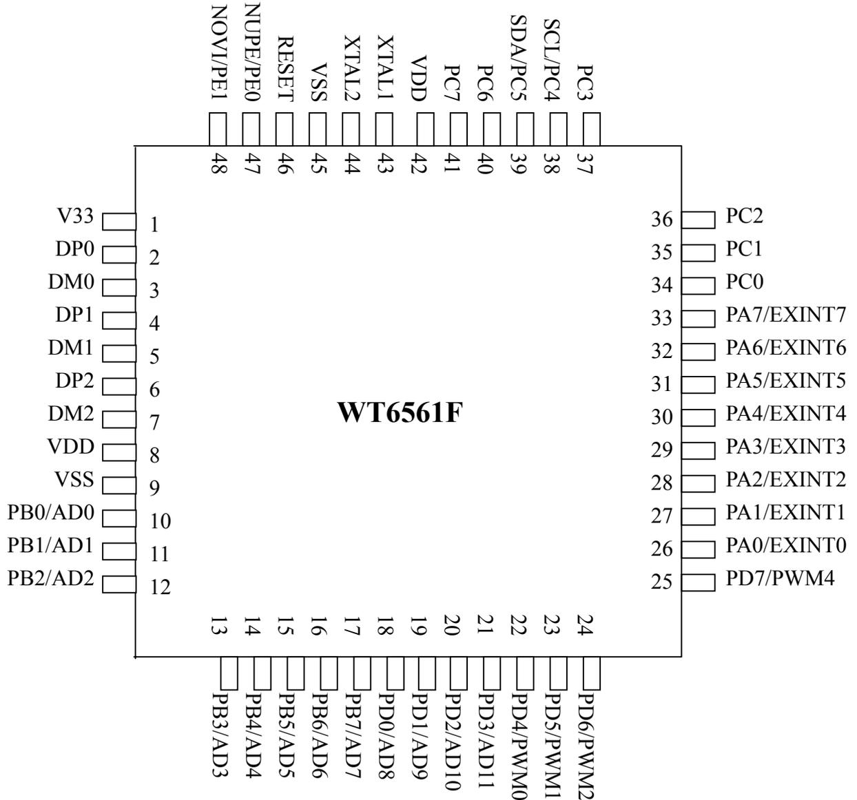
**Figure 1. WT6561F 48-Pin QFP Package**
