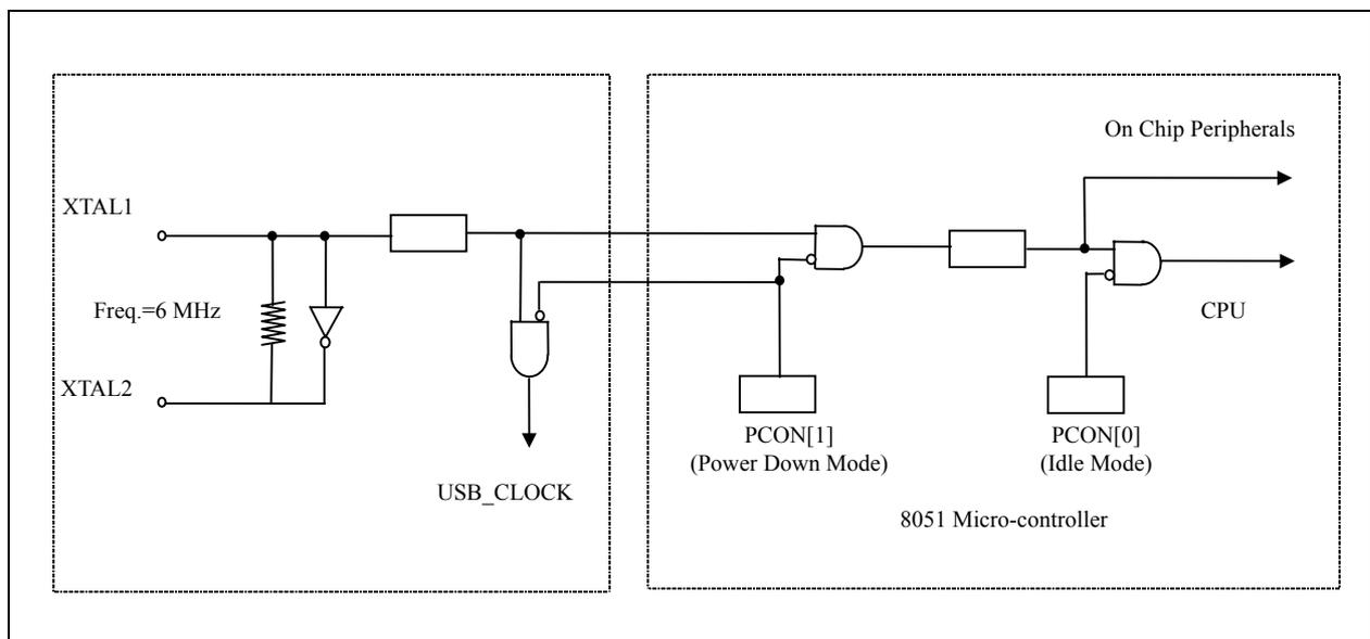
**Figure 4. Clock Circuit**
