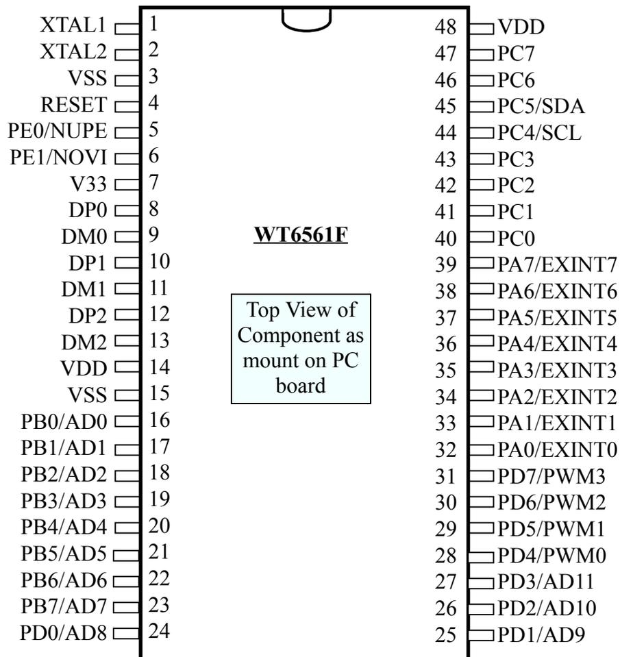
**Figure 2. WT6561F 48-Pin DIP Package**
