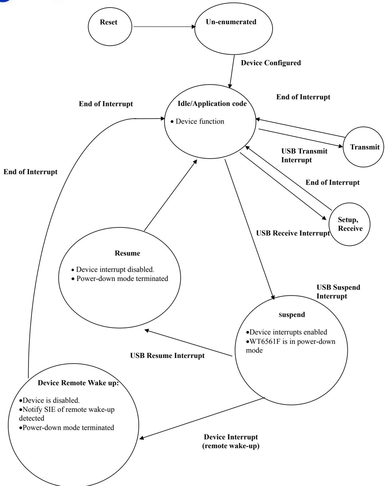
**Figure 7. Suspend and Resume State Diagram**
