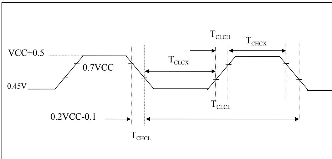
**Figure 8. External Clock Drive Waveform**
