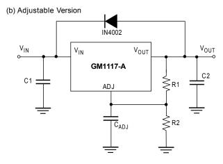
In the GM117 linear regulators, the discharge path is through a large junction, and protection diodes are normally not needed. However, if the regulator is used with large output capacitance values and the input voltage is instantaneously shorted to ground, damage can occur. In this case, a diode connected as shown above in Figure 1.
