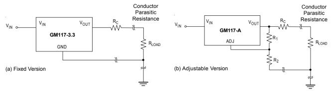
FIGURE 2<sup>(a),(b)</sup> Conductor Parasitic Resistance Effects are Minimized by this Grounding Scheme For Fixed and Adjustable Output Regulators
