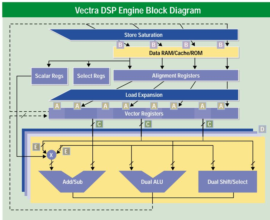
Figure 5. The Vectra engine's Vector/SIMD architecture is optimized for efficiency and performance
