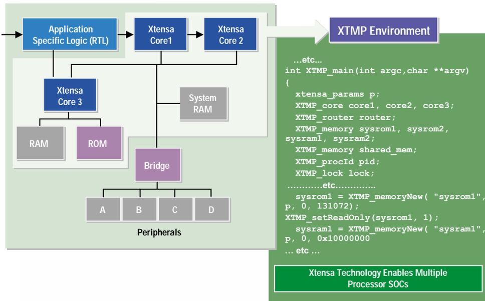
Figure 4. Xtensa Modeling Protocol (XTMP) environment for multiple-processor system simulation
