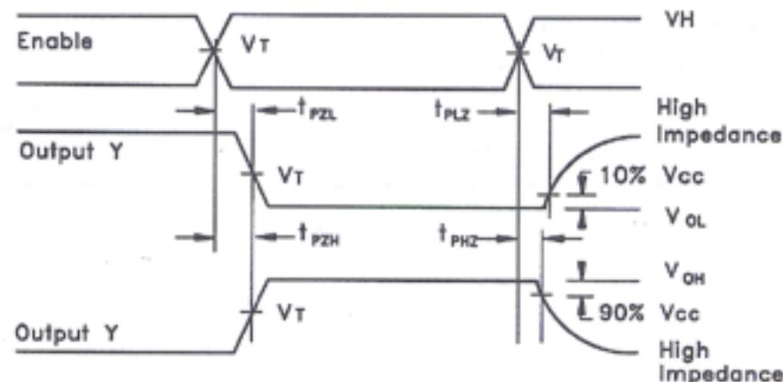
Input and Output Threshold Voltage:  $V_T = 50\% V_{CC}$  for HC, 1.3V for HCT,  $V_H = V_{CC}$  for HC, 3V for HCT
