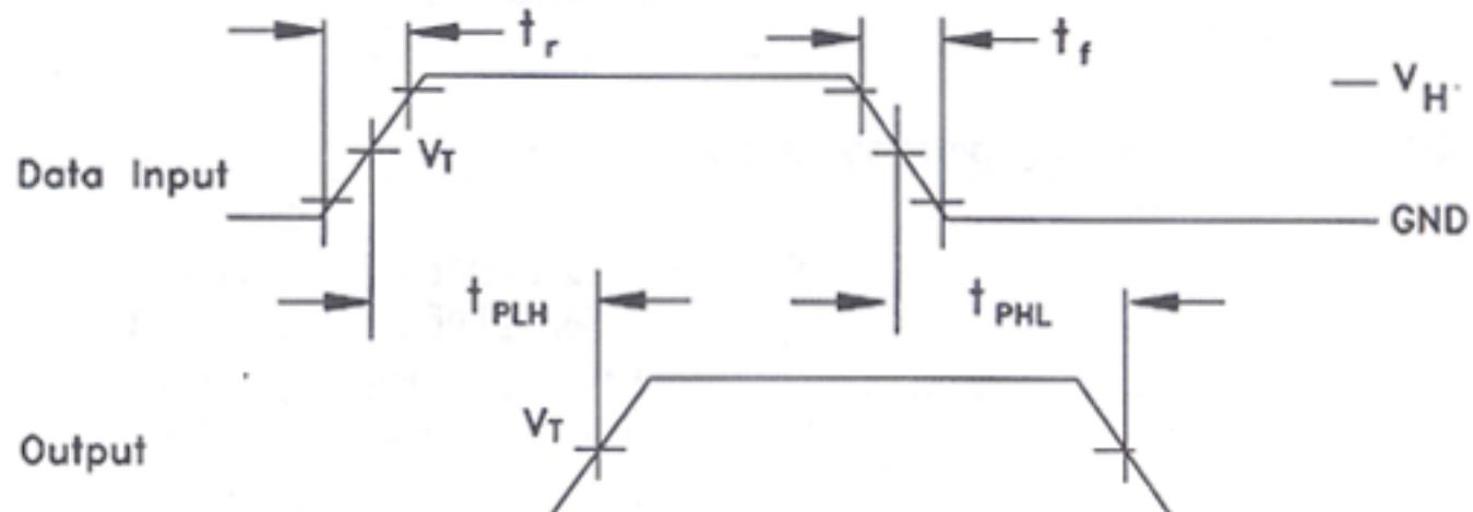
Input and output threshold voltage:
