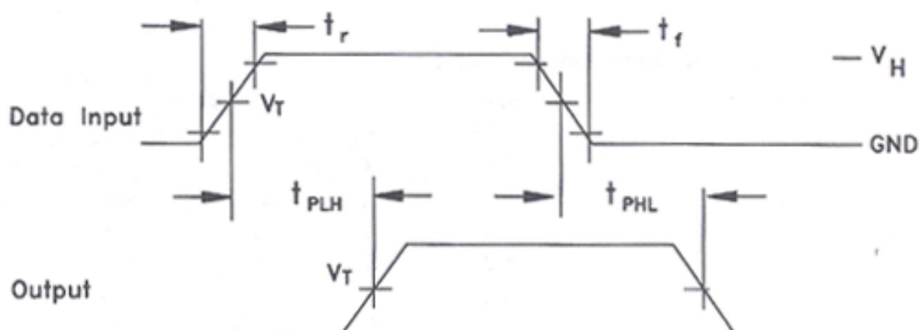
Input and output threshold voltage:
