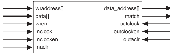
Figure 23. APEX 20KE CAM Block Diagram
